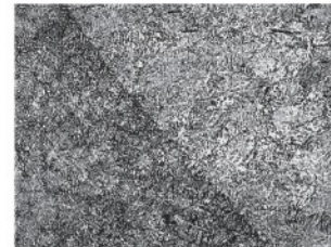
Figure 3: Acceptable microstructure in heat affected zone. (100X) (1)
