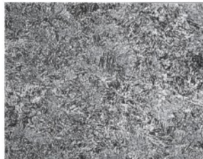
Figure 2: Acceptable microstructure after welding. (100X) (1)
